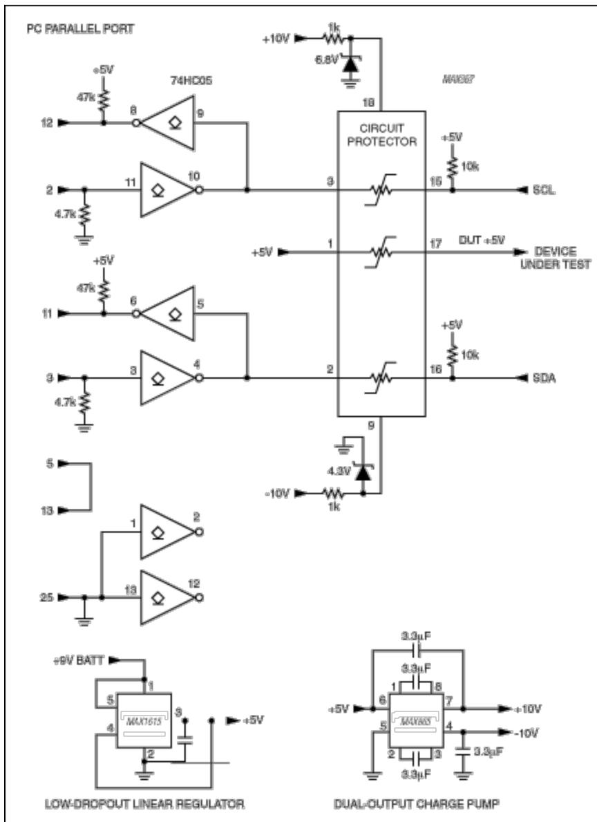
Figure 2. This parallel-port-to-I<sup>2</sup>C interface provides the open-collector connection to the I<sup>2</sup>C serial port mandated by the I<sup>2</sup>C specification. The MAX367 circuit-protector IC keeps voltages that exceed the supply rails from damaging the interface circuitry as well as the parallel port itself.
