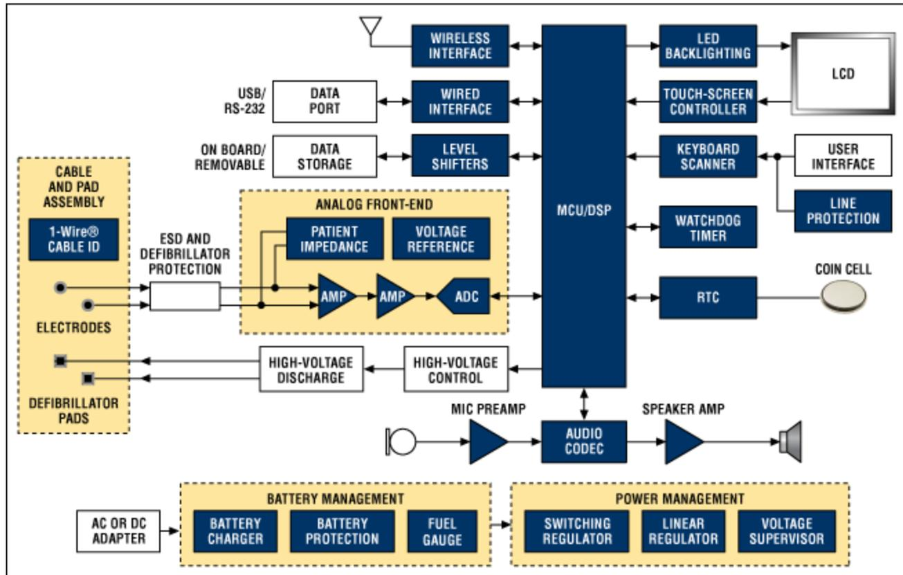
Functional block diagram for an AED device. For a list of Maxim's recommended solutions for an AED design, please go to: [www.maximintegrated.com/AED](http://www.maximintegrated.com/AED).
