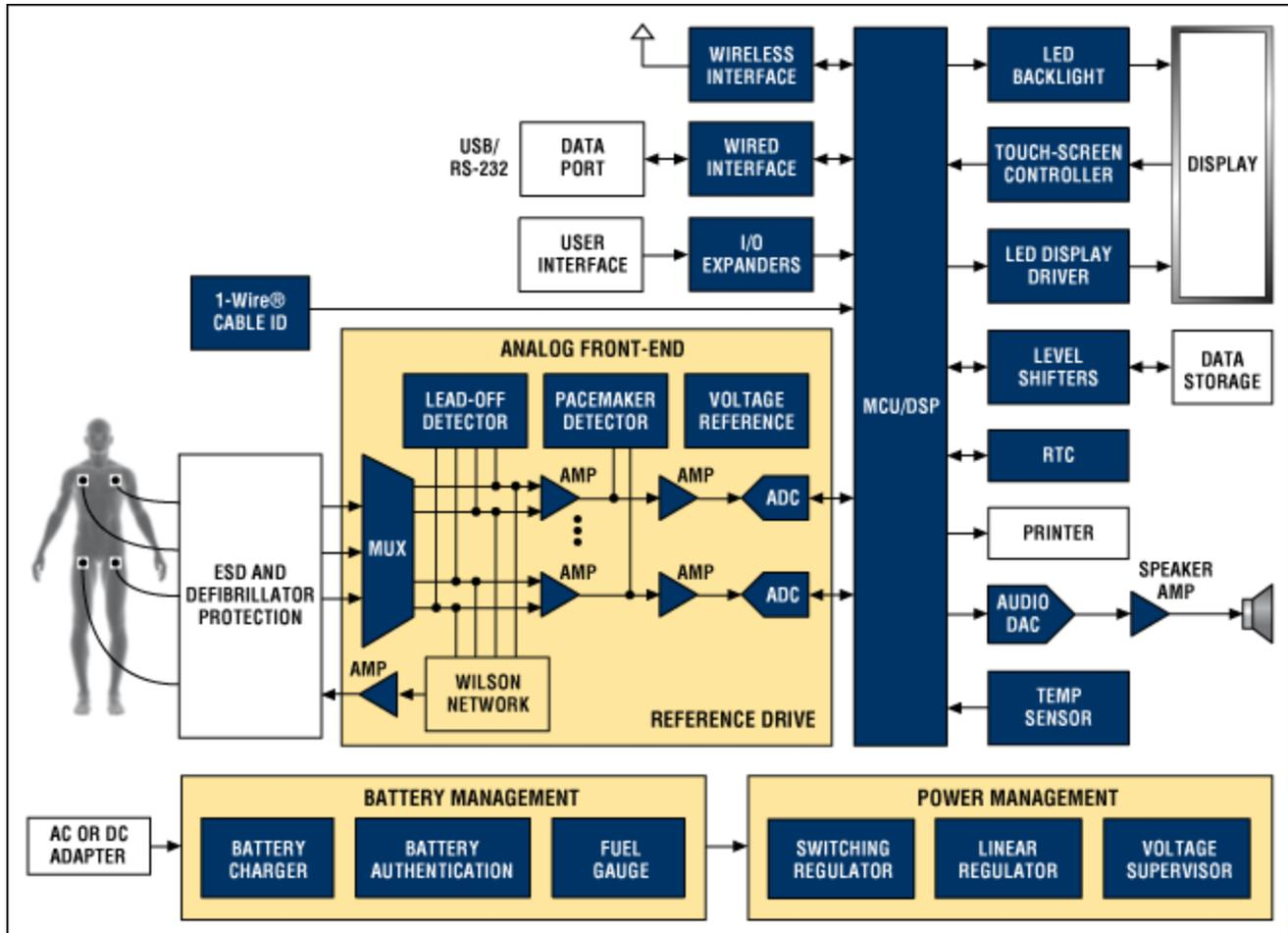
Full-featured ECG functional block diagram. For a list of Maxim's recommended solutions for an ECG design, please go to: [www.maximintegrated.com/ECG](http://www.maximintegrated.com/ECG).
