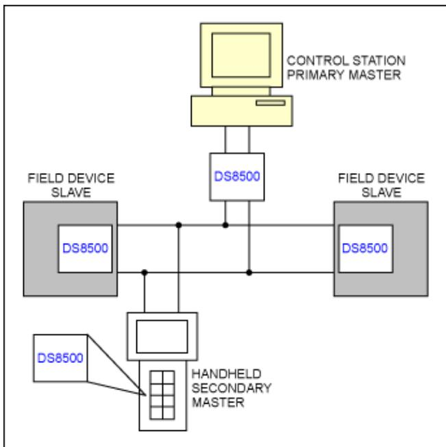
Figure 6. HART devices connections.
