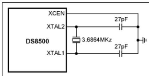
Figure 2. Crystal connection for the DS8500.
