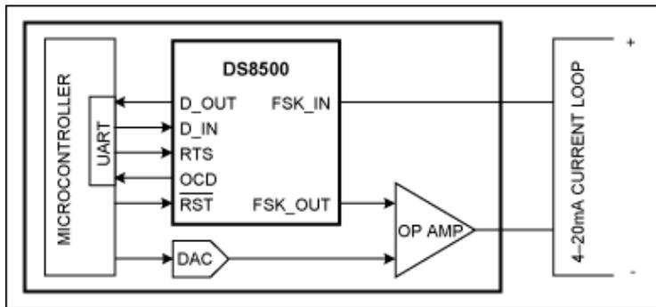
Figure 1. An intelligent process transmitter features the DS8500 HART modem communicating with a system microcontroller.
