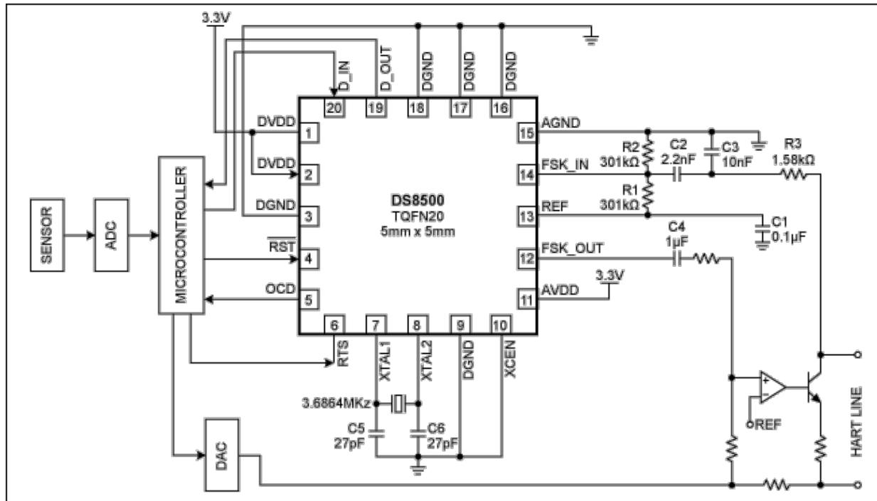
Figure 7. DS8500 on the slave side of HART communication. D\_IN receives data from the microcontroller's UART. D\_OUT transmits data to the UART. Active-low RST is the DS8500 reset. OCD is a carrier-detect signal that determines a FSK signal with a valid amplitude at the input of the demodulator.
