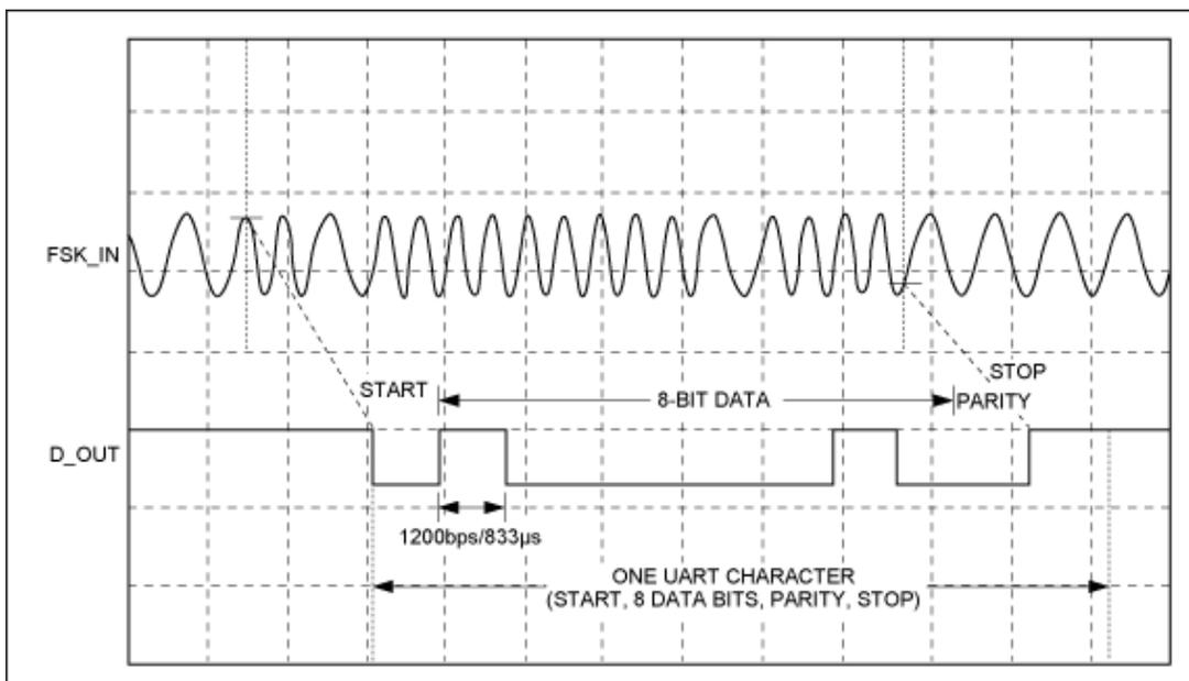
Figure 4. Demodulator waveform.
