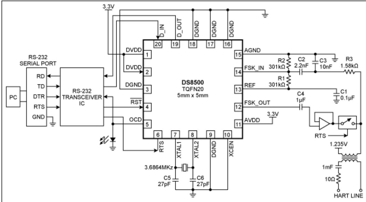
Figure 8. DS8500 on the master side of HART communication. D\_IN receives data from the microcontroller's UART. D\_OUT transmits data to the UART. Active-low RST is the DS8500 reset. OCD is a carrier-detect signal that determines a FSK signal with a valid amplitude at the input of the demodulator.
